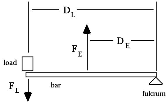
For all three classes of levers, the mechanical advantage is given by the equation below.
