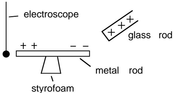
In this device, a charged glass rod is brought close to the insulated metal rod. Electrons move to the right leaving the left end positive. The styrofoam ball is neutral and moves right until touches the metal and becomes positively charged. It is then repelled to the left.
