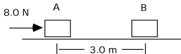
The work done on the box equals  $8.0 \times 3.0 = 24 \text{ N m}$  or 24 joules. If there is no friction, the box will accelerate. If the friction is  $-8.0 \text{ N}$ , the box will move at a constant speed. In both cases, the work done by the  $8.0 \text{ N}$  force is 24 J.
