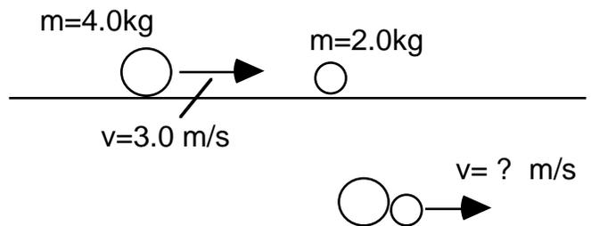
The initial total momentum is  $4.0 \times 3.0 = 12$  kg m/s. The final total momentum = 12 kg m/s. The final velocity = 2.0 m/s since the total final mass = 6.0 kg.
