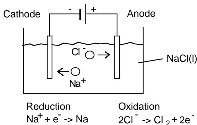
There are many practical problems that must be overcome in order to run this cell. The melting point of NaCl is 800°C and the sodium and chlorine must not come in contact or an explosion will occur.
