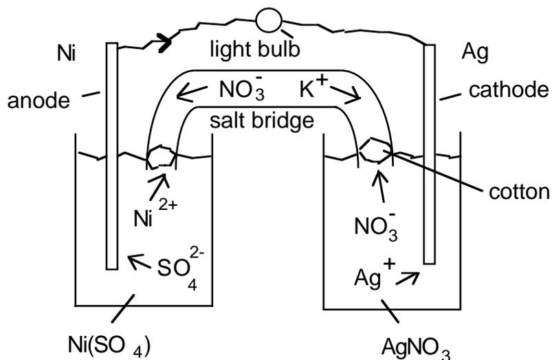
2)a) Ni, b) Ag, c) Ag, d) Ni, e) Suitable solutions : Ni half-cell,  $\text{NiSO}_4$ , Ag half-cell,  $\text{AgNO}_3$ , salt bridge,  $\text{KNO}_3$ .
